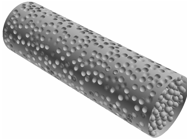
Figure 1: Particle configuration for the simulations of the present study. The side wall of the duct is roughened to avoid exiting the higher velocity region near the tube wall
